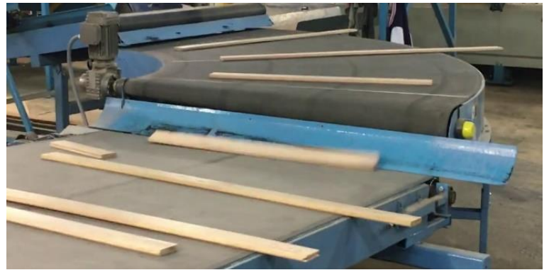
90-deg. Flat-Turn used in wood furniture production
