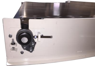
90-deg. Flat-Turn used in wood furniture production
