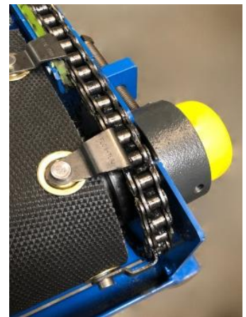
Chain Attachment and Sprocket Detail (Chain Cover Removed)
