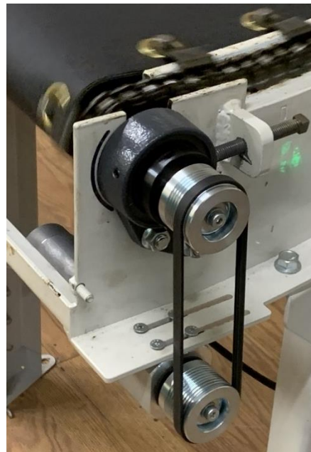
Drive Configuration (Chain Cover and Timing Belt Cover removed to show detail)
